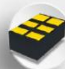
DFN1610-6L 2A-200A 3.3V - 30V 1.6*1.0*0.55mm
