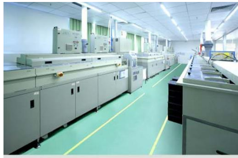
去溢料工序 DEFLASHING
