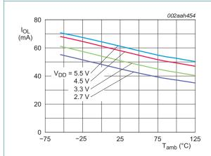
Fig 22. LOW-level output current on SDA pin versus temperature;  $V_{OL} = 0.4 \text{ V}$
