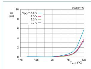
Fig 20. HIGH-level input current versus temperature; digital pins
