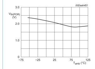
Fig 24. Power-on reset threshold voltage versus temperature; rising  $V_{\text{CC}}$
