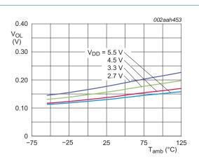
Fig 21. LOW-level output voltage on SDA pin versus temperature;  $I_{OL} = 20 \text{ mA}$
