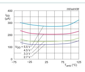
Fig 15. Average supply current versus temperature; I<sup>2</sup>C-bus active
