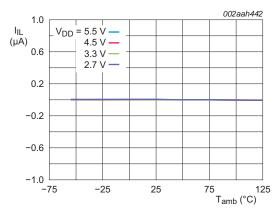
Fig 19. LOW-level input current versus temperature; digital pins
