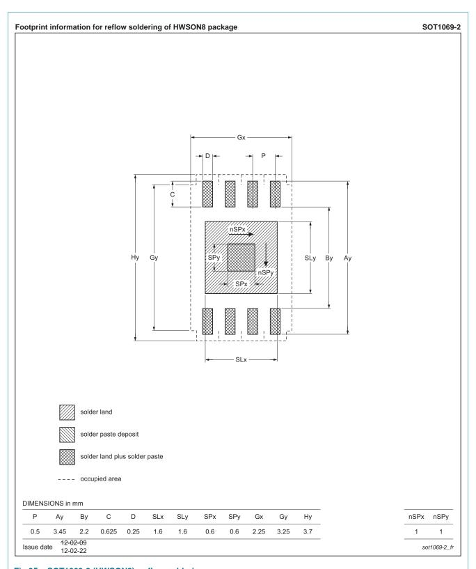
Fig 35. SOT1069-2 (HWSON8); reflow soldering
