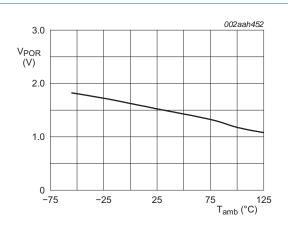
Fig 25. Power-on reset voltage versus temperature; falling V<sub>CC</sub>
