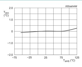
Fig 23. Temperature accuracy versus temperature;  $V_{CC}$  = 2.8 V to 5.5 V
