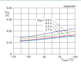
Fig 17. LOW-level output voltage on OS pin versus temperature; I<sub>OL</sub> = 4 mA
